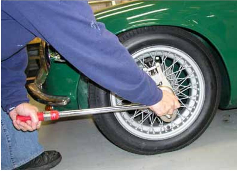
Tightening the spinner is just the reverse, but is infinitely more satisfying. Why? Because it is in the tightening process that the tool proves its value. Adjust the torque wrench to 220 pounds-feet and tighten. What is so special? Well, there is no chance that you will ruin the body or paintwork of your precious Elite and you will never accidentally hit one or more spokes and ruin a wheel. Note: On the front wheels, you may need to chalk the wheel to keep it from spinning.
